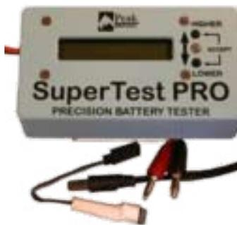
separate 12 volt power supply and can be programmed to cut off from 1.0 -14.0 volts in 0.1 volt steps at discharge rates of 125, 250, 500, 750, 1,000, 1,500 or 2,000 MaH. So \$100 later I had my new SuperTest Pro discharger.
