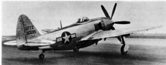
XP-72 No.2 (43-6599) with six-bladed contra-rotating coaxial propeller.
