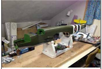
To finish off the build, I installed Futaba RX, HiTec servos throughout, dual Futaba switches going to the RX, and both powered by 2s 3000mah LiFe batteries for a full redundant system. An aircraft this big with this many servos, it's nice to have a backup plan. For power I used two Turnigy .46 size electric motors with Turnigy
