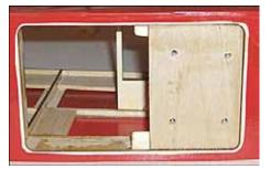
flush with the bottom of the fuselage. Also, strips cut from 1/8" x 1" hardwood were used to reinforce the fuselage side and also to provide additional thickness for the blind nuts. Note: the new Deluxe Telemaster 40 kit includes an optional float strong point.
