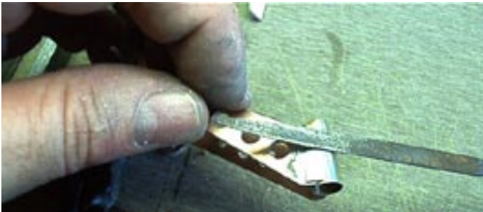
Using a file, clean up the solder joints.
