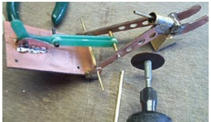
Solder the upper support bearing on.
