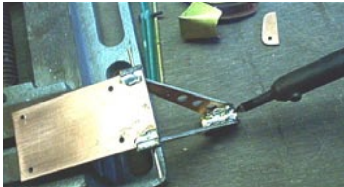
Solder the back side of the yoke support tube to the forks, use plenty of solder.
