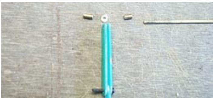
Using a file, clean up the solder joints.
