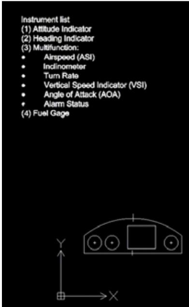
The instrument requirements for VFR flight (day) are contained in the FAA's "Code of Federal Regulations, Sec. 91.205. In so far as possible, I wanted the Laker's instrument panel to contain a set of required instruments, including an airspeed indicator, altimeter, magnetic direction indicator, and fuel gage. Searching
