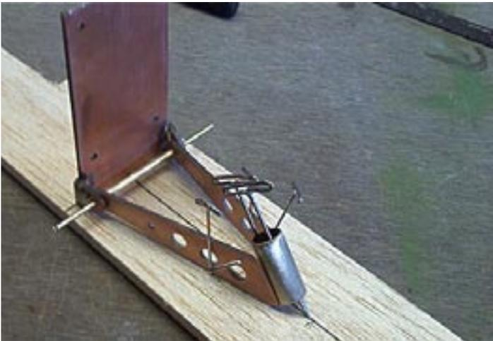
Next glue the back plate to the jig with medium CA and add whatever pins are needed to secure the parts.
