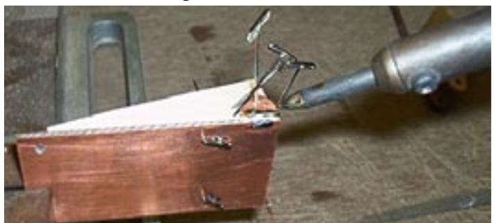
Again use pins to hold the parts down and add two small drops of solder to the parts.
