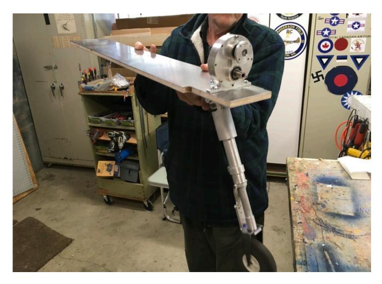
Although the Nose Gear is not completely finished, even with the temporary struts and bracing there are no clearance issues. Next, we locate the Torque Plate mounting holes.
