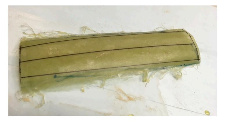
The process worked well. The resin did not stick to the tape. I got perfectly contoured doors.
