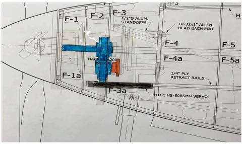
Jim has enough of the parts completed we were able to do a partial install and test to see if we had the clearances correct. There is very little room in the lower half of the fuselage for the Nose Gear due to the thickness of our Torque Plate and the Gearbox size. We had spent a fair amount of time measuring things and making sure we had everything in the correct place.
