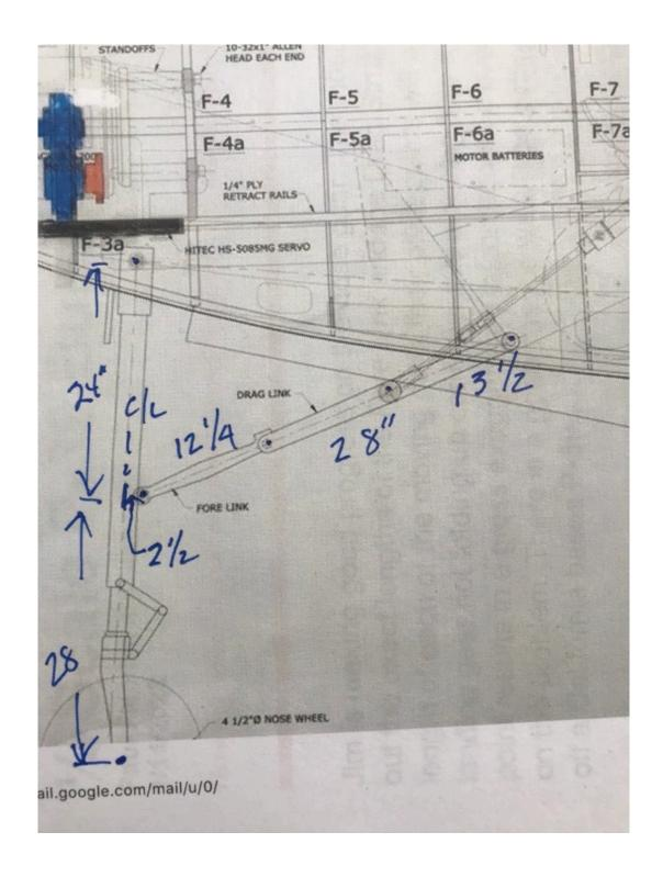
In the mean while Jim has started building the nose gear. He has completed the pivot and rotating sleeve assembly. This joint allows the nose gear to pivot and retract and allows the strut to be swiveled for steering.
