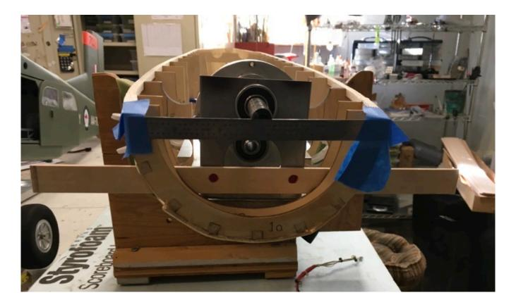
We taped a steel ruler across the lower fuselage half to locate exact horizontal plane and installed temporary supports. A brass tube was inserted into the propeller shaft tube and a laser line was projected from the side along the fuselage top and brass tube to get the vertical plane. (Sorry that didn't photograph well.) Once all the temporary supports were in place, we plotted the foundation bolt locations. We removed the
