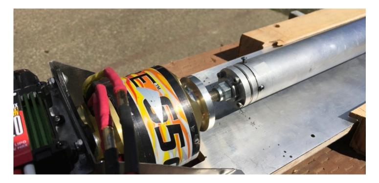
To allow the Torque Plate to roll slightly forward as thrust is increased, we used ½ PVC pipe as rollers. Our sliding mount seemed to work fine for simple running. I am certain
