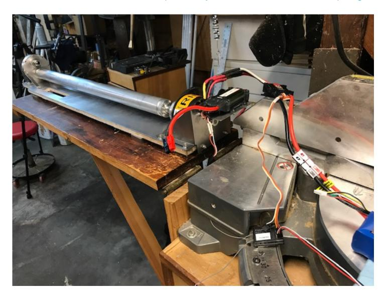
The first run was conducted using a 4s battery. Things went smoothly although the thrust bearing retainer nut on the gearbox loosened. We did notice a slight amount of wobble on the shaft coupling on the motor end. The drive tube is bonded to the shaft coupler we
