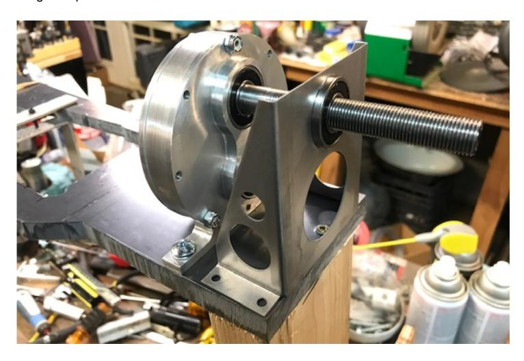
While waiting we finished the design of the nose gear. We had a couple of false starts on the actuator assembly. We first used a Clippard pneumatic cylinder thinking we needed about a four inch stroke. A problem was encountered was while folding the For Link and the Drag Link swing in two conflicting arcs and as they pass through the
