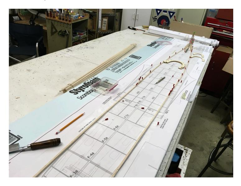
This fuselage splits and identifies top and bottom of each individually numbered frame. Example F-1 and F-1a, everything that has a letter after the number is on the bottom half of the fuselage. It is a very simple easy to follow method.
