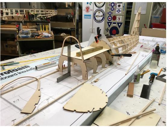
I have been planning to finish the aft upper fuselage, but discovered I am missing a couple of critical parts for installing the horizontal stabilizers. It is my intention t get the flight control linkage installed before I sheet the tail. That is all for now, videos in the works.
