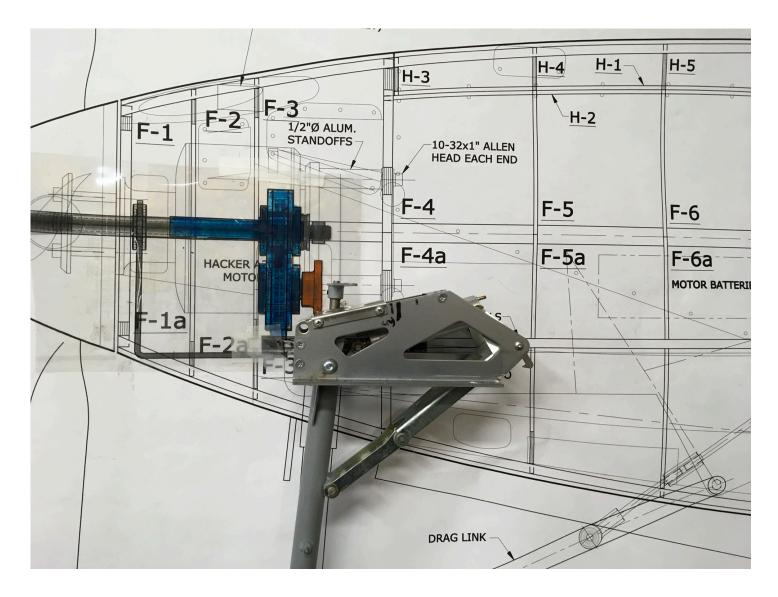
Since the actuator and steering arm were simply not going to work we decided to mount the nose gear to the bottom of the Torque Plate. How to pivot the gear leg up and steer via cables were easy. Building pieces to make this work were straight forward enough, but how are we going to get it to move. The plans show a type of gear retraction parts. I think this might be a Century Jet Unit. As shone nose gear installed which roughly duplicated the way Bell Aircraft did it.
