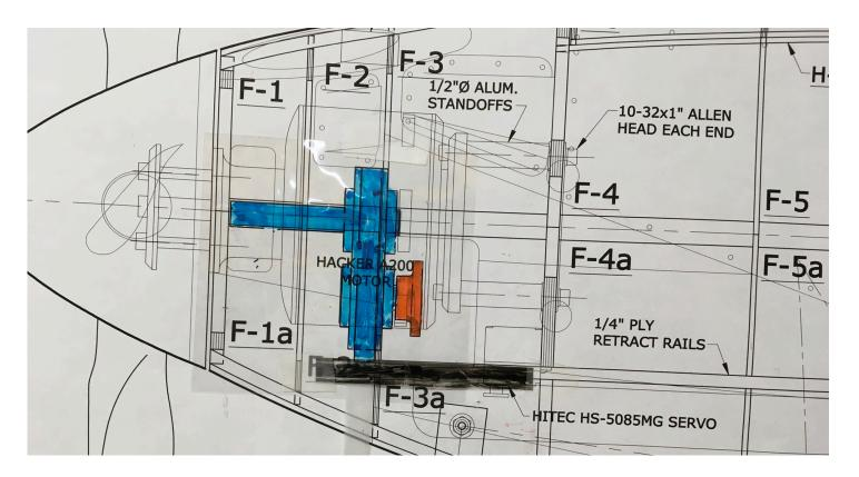
Using a full scale Gearbox and Torque Plate template over the fuselage frames we could easily see the material that needed to be removed and plot the cutting lines.
