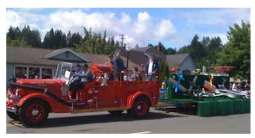
Is a 1936 General it has a 500 gpm Northren rotory gear pump. It has a 6 cyclinder Hercules with 94 hp. It was in service from 1936 till 1948 In Glass Glow MO. They paid \$5200.00
