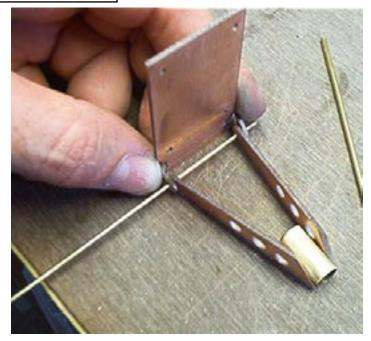
I'm using .063 brass rod for the pivot, the 3/32" brass tube fits right over it. I'm checking the fit of the brass rod, once it's satisfactory cut a length of 3/32" tube to fit in the middle, do not solder it in yet.
