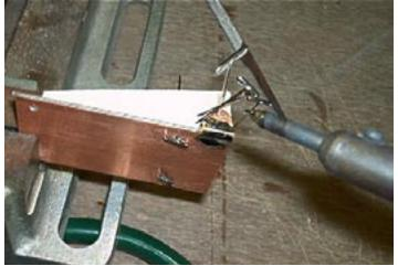
Set your 1/8" brass angle on the solder and then rest your soldering iron on it and it will draw it right down to the parts. Use some solder on the outside edges also to strengthen them.
