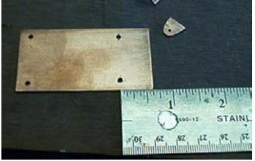
Drill your mounting holes in back plate. Measure 5/8" from the bottom for the lower holes, this will give you clearance from the pivot axle so that you can actually insert the mounting screws when the time comes.
