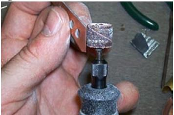
Sand the ends of the supports to the proper angle, make sure to orient them correctly and make sure you make one left and right side!
