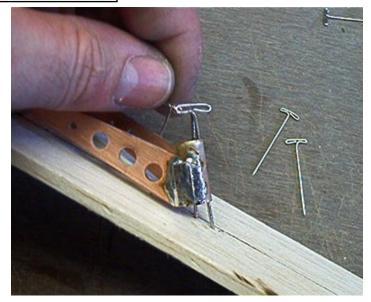
I used some small strips of .005 brass to cover the joint at the end of the supports, use plenty of solder, you can file it down in a bit!
