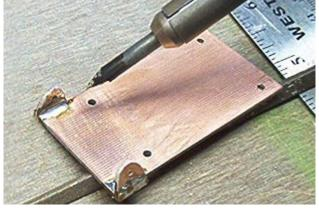
Remove the back plate from the jig and solder the inner joints of the pivot bearings.
