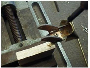
Remove the yoke from the jig and solder the inside of the forks to the top piece.
