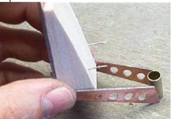
Check the angle and sand as needed to get the proper angle.
